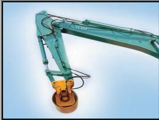
Fig-E2: Slope Vibratory Roller
