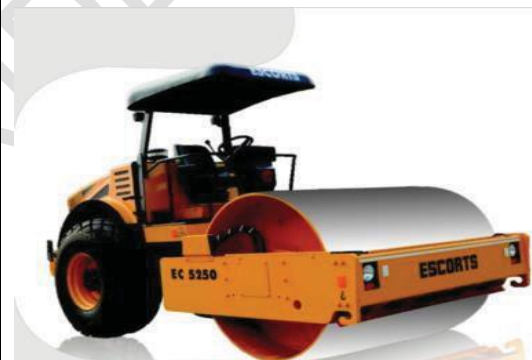
Fig-E9.2: (Available in Standard, Drum& Pads + Drum type & used for better gradeability & breaking clods)
