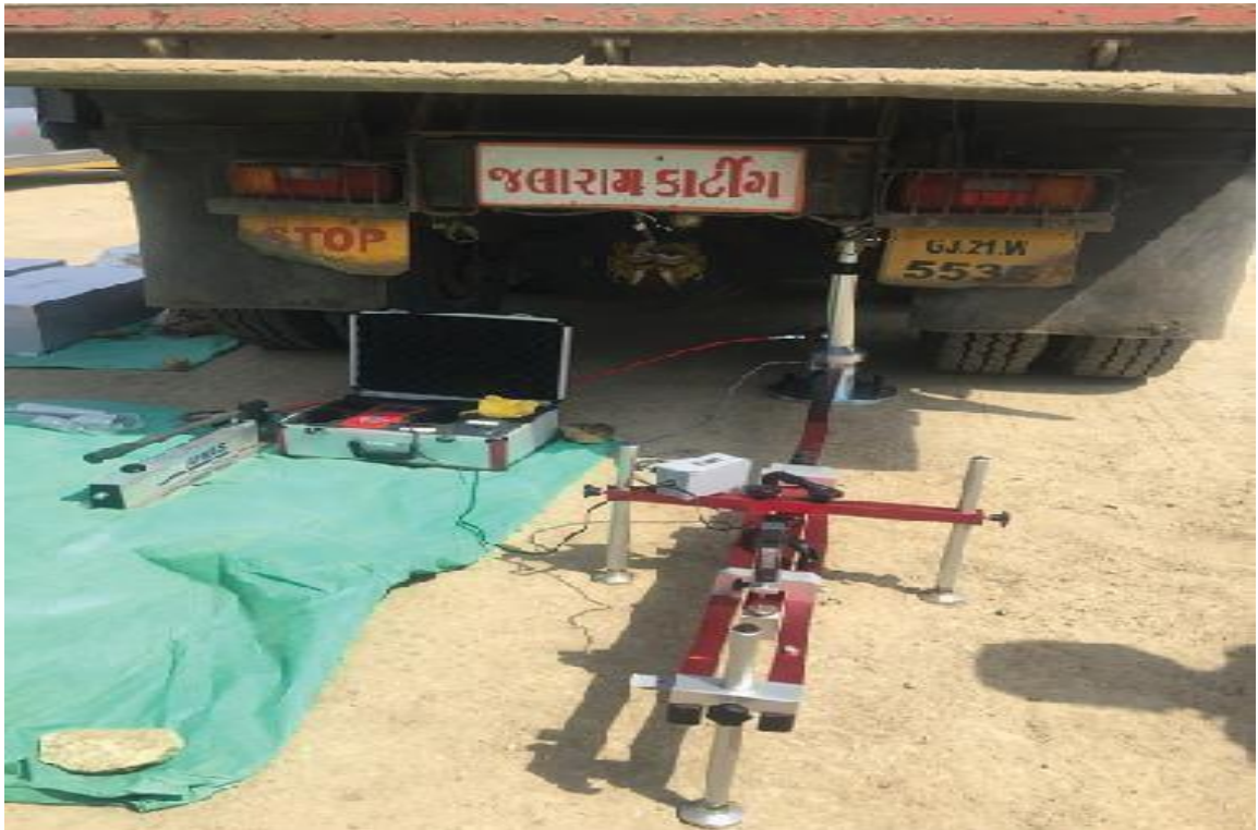
Fig-H 6: Ev 2 Measuring Equipment
