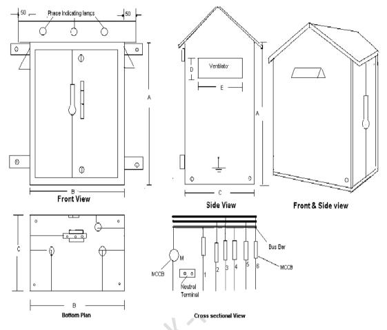
Note: Separate Terminal bar to be provided for neutral connection.
