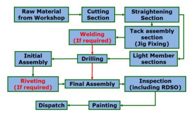
5.4. Considering the length and height of span, jigs and fixtures shall be used to guide and support drilling of holes and fixtures during entire fabrication work assembly of components, before riveting / welding of components.
