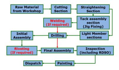
5.4. Considering the length and height of span, jigs and fixtures shall be used to guide and support drilling of holes and fixtures during entire fabrication work assembly of components, before riveting / welding of components.
